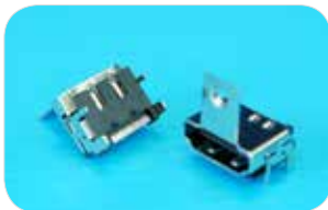
CHDM-P19RS30-H3 (H5) ▶ R/A, SMT, With Flange H*W=10.3mm*7.5mm, ▶ Without Post (H5=With Posts)
