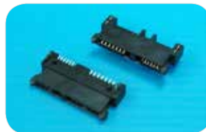
CSAT-F13RS30-GA ▶ Female, R/A, SMT, Standard Type, H=4.50mm
