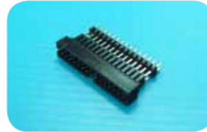
CB20-2XXVDG0-1L ▶ Pitch 2.0mm, 2*XXP, Vertical, ▶ DIP, High Profile
